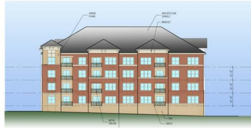
4 SOUTH ELEVATION (SOUTH BLDG) SCALE: 1/16" = 1'-0"
