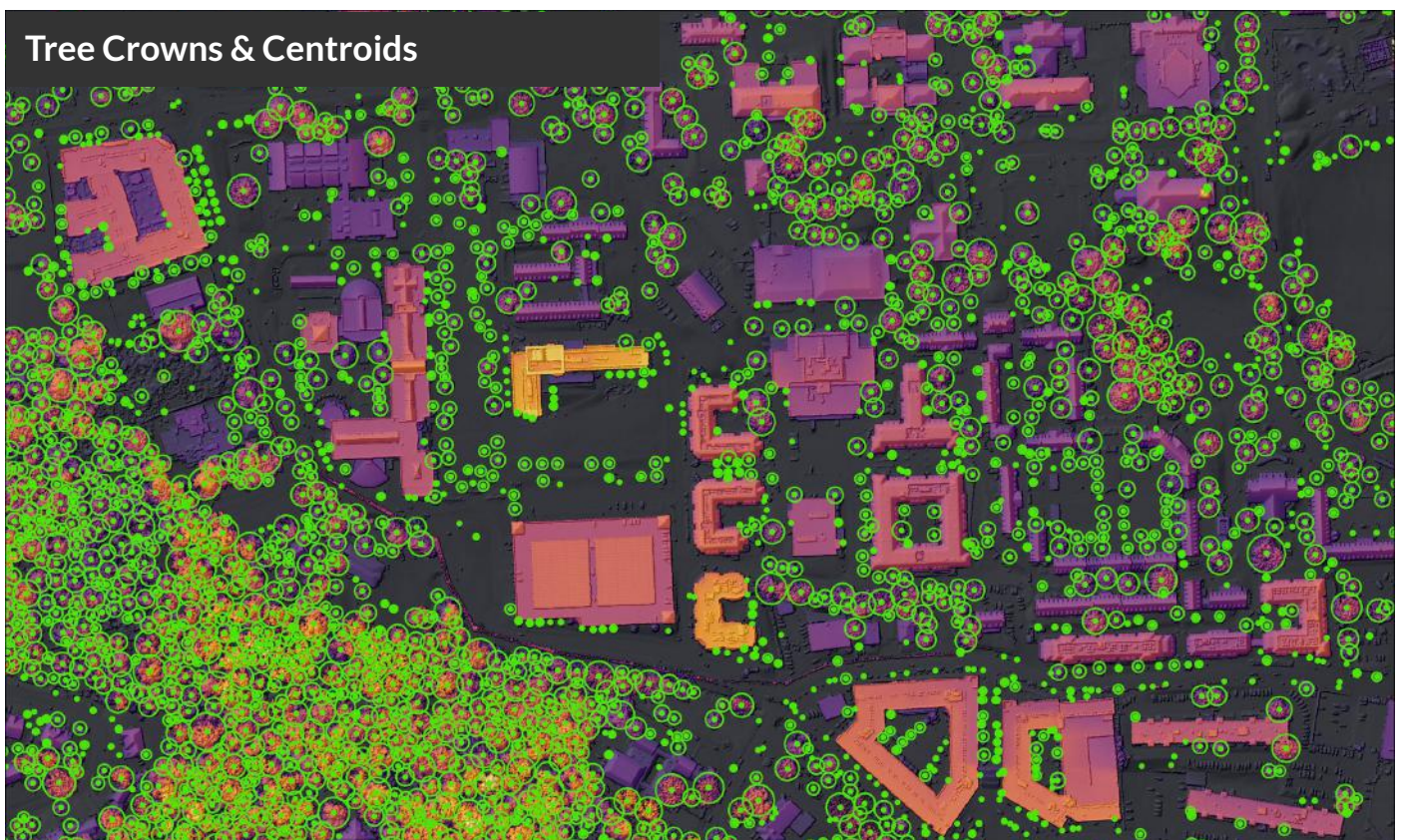
Figure 3. Tree centroids (dots) and tree crowns (circles) mapped from the 2020 LiDAR. Tree mapping from LiDAR involves finding relative high points for each tree, then tracing down until a height inflection point is reached, marking the edge of the crown. This approach to individual tree mapping is most accurate where there is a clear differentiation in tree crowns and is less accurate in forested stands where crowns may overlap.
