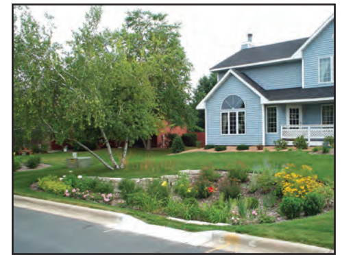
Typical example of a rain garden
